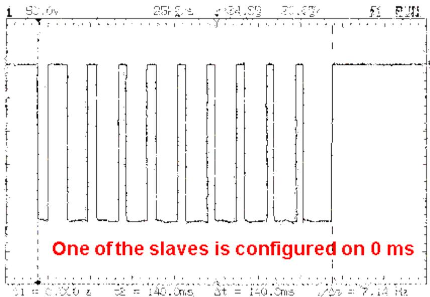
This curve shows only 9 pulses on a current loop for a SFLS of 10 flashes !
